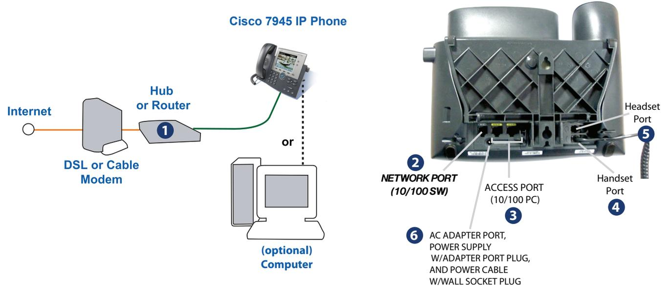
**Step 1:** Connect the network 10/100 SW port 2 to an available port on your switch or router using an Ethernet cable. 1
